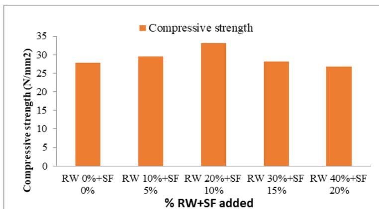
**Fig 1:** Compressive strength for 28 days strength
