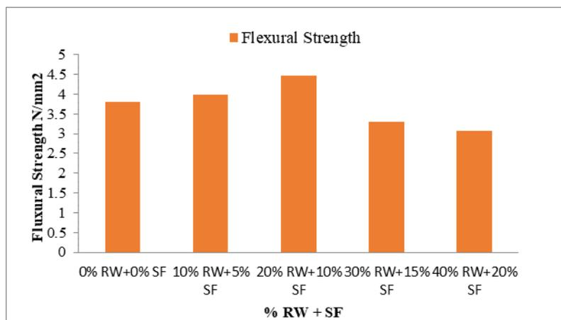
Fig 2: Flexural strength for 28 days strength
